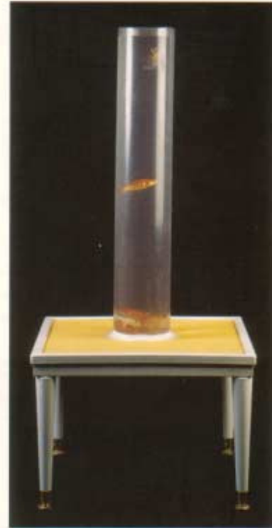
StoGuard has been tested in accordance with AATCC-127 (modified), Water Resistance: Hydrostatic Pressure Test, and resists water penetration for months. Ordinary housewraps and building papers, depending on brand or type, measure water resistance in hours, and in some cases, allow water penetration within the first few minutes of exposure.
